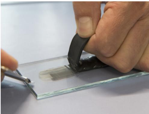
*-> Pull off the adhesive bead and assess the fracture pattern. If there is a cohesion break in the adhesive, the adhesion to the substrate is perfect.*
