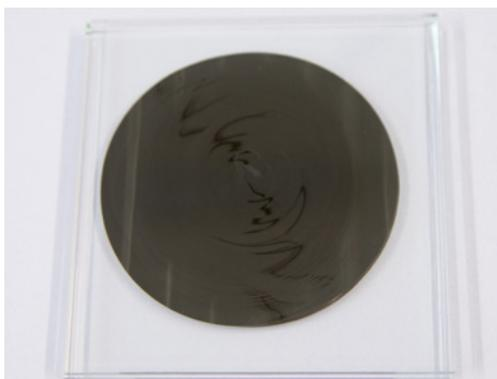
*Glass plate test – Expected mixing pattern
