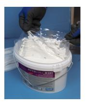
After opening the container, remove the packet of silica beads and then, starting at the container edge, pull off the film and remove any hardened material if necessary (do not stir in!). If the adhesive is not needed in its entirety, save the silica bead packet and the film for resealing later.
